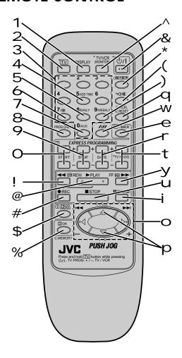
Buttons with a small dot on the left side of the name can also be used to operate your TV while holding down the **TV** button.  $\square$  pg. 54
